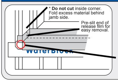
3. Pre-split approximately 1" of the 40 mil waterproof flashing membranes release film for easy removal. Press membrane into sill, jamb and inside corner. Fold excess material from inside corner toward jamb side. Staple into place on bucks and jambs. Peel at pre-slit and adhere to jamb, sill and sill face. Roll with J-Roller.
